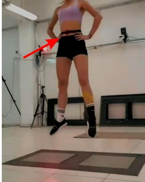
Figure 1. Illustrative image of accelerometer positioning.
